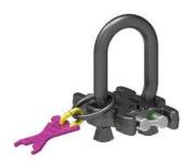
Master link with an integrated shortening option specially developed for the 4mm ICE lifting chain. Can also be used as a single leg (ICE - Endlink 7905039 assembled at the end of the chain sling as a stop device). With the pressing of the locking bolt the chain crucifix is freed and the chain can be mounted and respectively be adjusted to the desired length. Ideal for small loads up to 1120 kg (in a 2- leg application).
