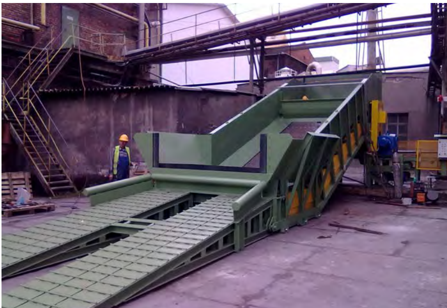
RUD unloading ramp system for truck unloading into the conveyor.
