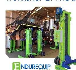
Our workshop lifting and handling solutions include Endurequip Portalift, which are the only portable heavy vehicle hoists made in Australia.
