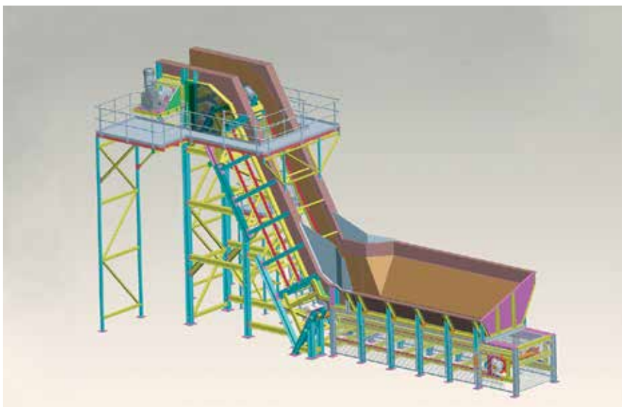
RUD apron feeder provides storage, metering and elevation of the product.
