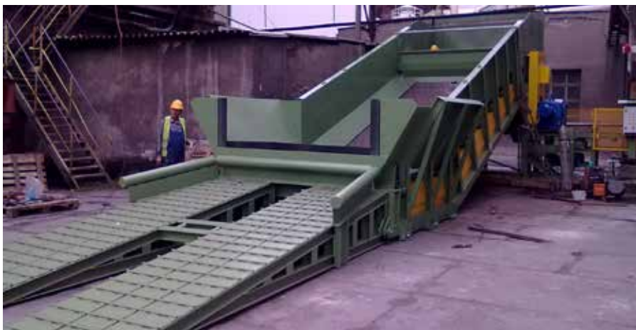
RUD unloading ramp system for truck unloading into the conveyor.
