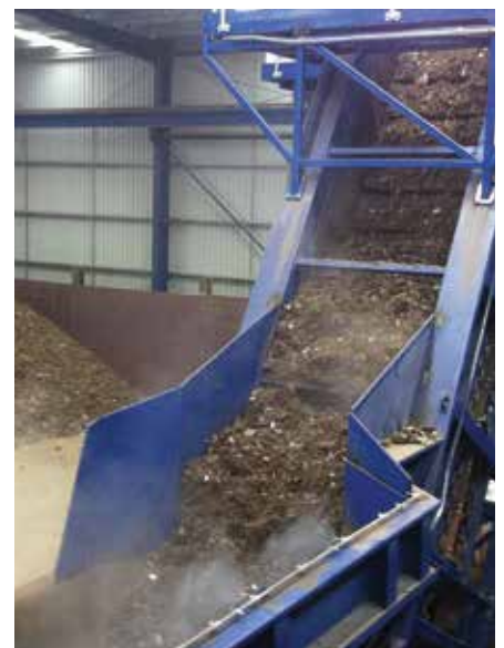
A RUD tumble back apron feeder processing flock ASR material.
