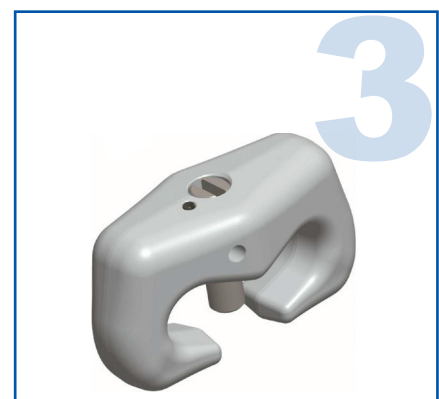
Step 3 To open, rotate the locking bolt again in a clockwise direction until you hear a click (now the pin is unlocked)
