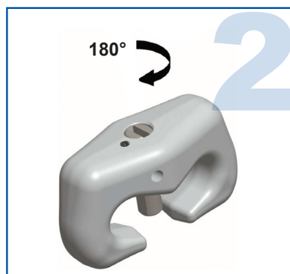
Step 2 Rotate the locking bolt in a clockwise direction until you hear a click (now the pin is locked).
